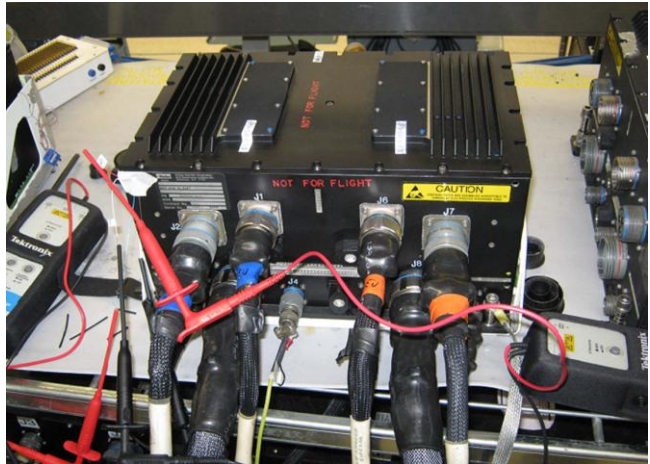
Figure 7. Power drive electronics (PDE) unit
