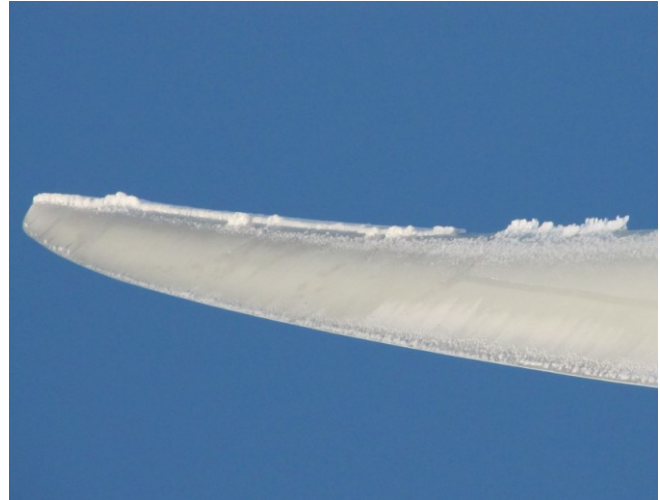
Figure 2 Icing on Wind Turbine Blade
