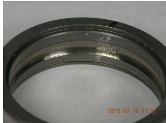
Figure 10. Example Outer Race Fault
