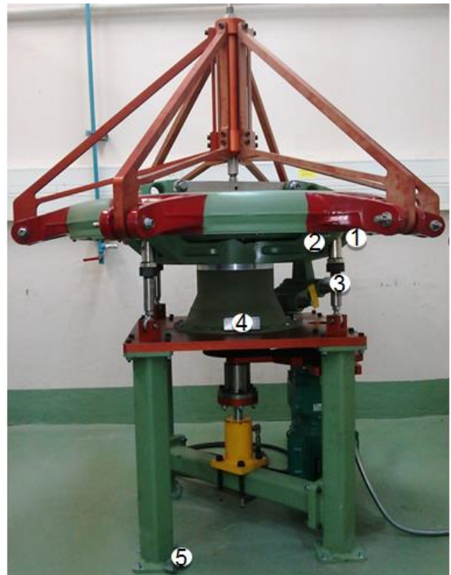
Figure 9. Full scale test rig and sensors locations
