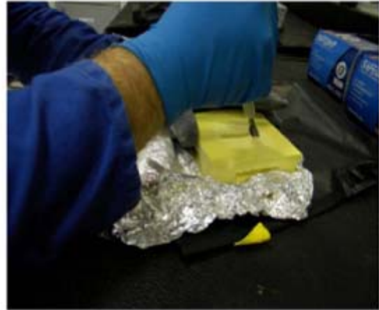
Figure 8. Peeled-Off Binder-Rich Layer
