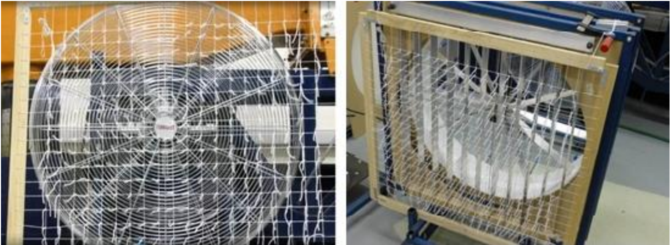
Figure 3: Flow vortex behind fan (left) and straightened flow with aerodynamic element (right)
