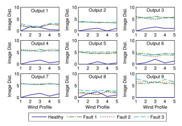
Image distances of the change signatures in the proximity of the third mode for the healthy and 30% damaged blade by each of the nine blade output locations
