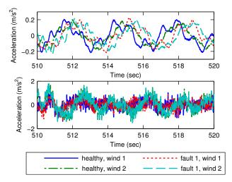
Acceleration of the tower at location 7 (top) and the blade at location 7 (bottom) after the brake maneuver is performed
