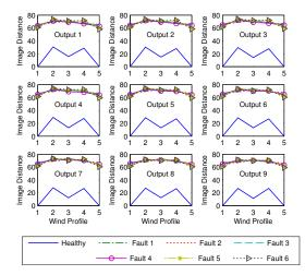
Image distances of the acceleration time histories at 9 output locations of the tower obtained for the healthy tower and a 5% damaged tower with five different wind profiles having a mean speed of 12 m/s
