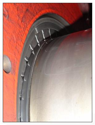
The space between these bearing rollers is too small to allow enough room for the borescope camera.
