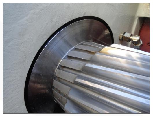
An example of a bearing with an oil dam plate blocking borescope camera access.
