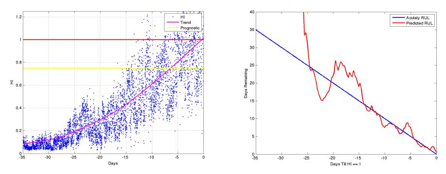
Fault Starts to Prorogate @-25 Days, Can See RUL Drop: Fault Sensitive to Load: Only Had RPM Used Nominal Power Output For RUL RUL Based on Operational Hours: Wind Does not Blow All of the time Calendar time? About x2, about 50 days
