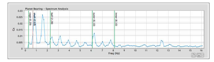
Why the Elevated CI? Engineering View Show Outer Race Fault/Ball Fault Subsequent Bore scope Confirmed
