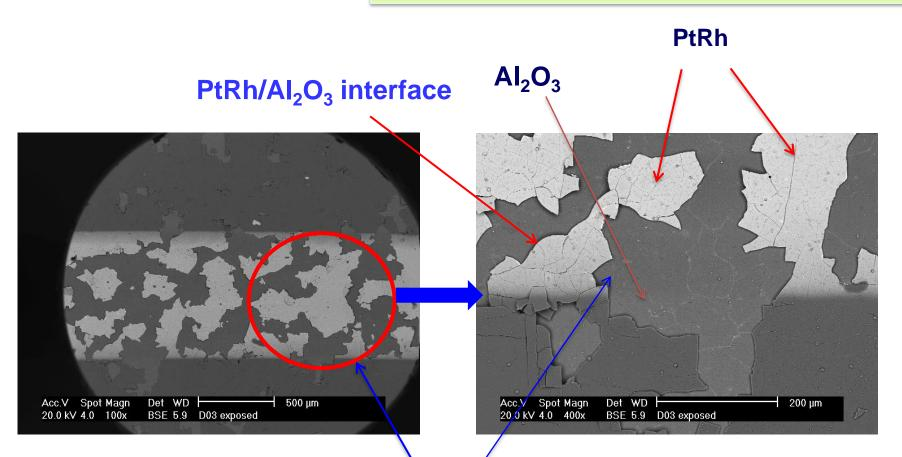
Sensor microstructure after thermocyclic testing followed by exposure to atmosphere for 12 days (SEM-BSE mode): Pt-13Ru leadout track delaminated.
