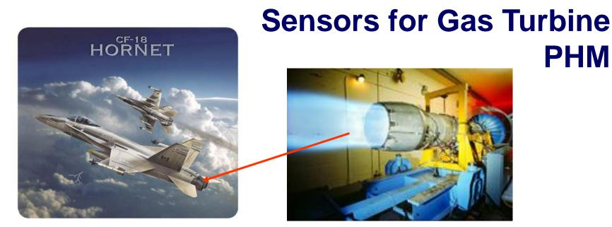
Sensors are needed for real-time monitoring of temperature, stress, fuel blow out, combustion instabilities, noise and  $NO_x$  emission etc.
