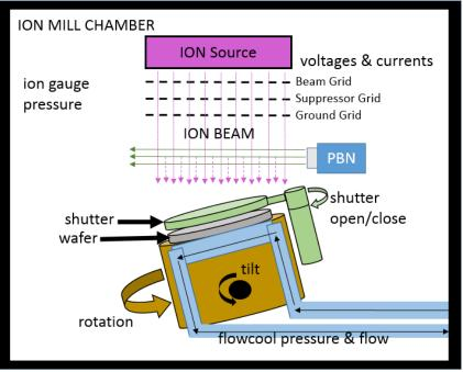
Figure 2. Wafer and ion mill etching process.
